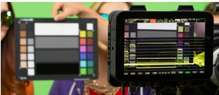
**Wave Form Monitor:** The wave form monitor can be used in conjunction with the large gray scale chips to help set exposure in pre-production. The values of the large gray square should match the values mentioned above.
