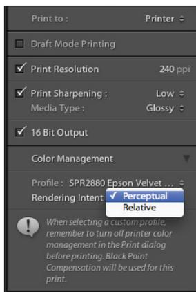
printing from Photoshop, you have to be careful to do this or the profile and printer driver will both try to manage color, and the resulting print will not be very pleasing or accurate (and won't even merit hanging on your refrigerator).
