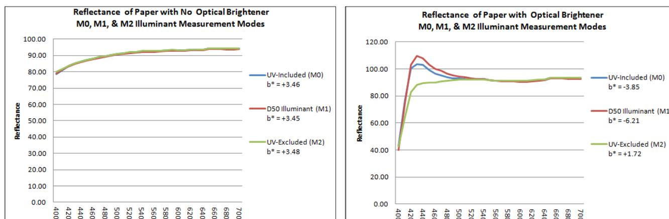
This chart clearly demonstrates the effects of three different illumination conditions on the same paper with and without optical brighteners.
