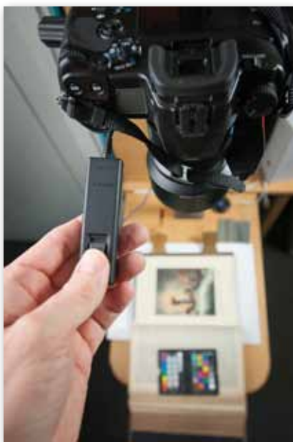
Vertical camera setup using a column from an old enlarger..
