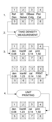
NOTE: The print parameters are setup in "Unit Configuration" Section 8.
