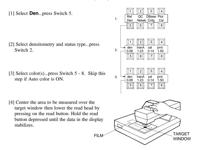
**NOTE:** A circular groove located on the light table is provided for holding disc type film. Simply position the disc into the groove and turn the disc until the desired frame is centered over the target window.
