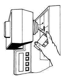
**NOTE:** When using an air can turn the unit on it's side and try to keep the air can upright, to avoid contamination.
